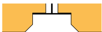
Shiplap and chamfered edges RST for thicknesses 25 - 35 mm with T24 profile RST35 for thicknesses 25 - 35 mm with T35 profile
